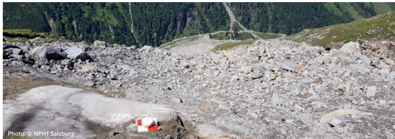
Installation ground control points (GCPs).
